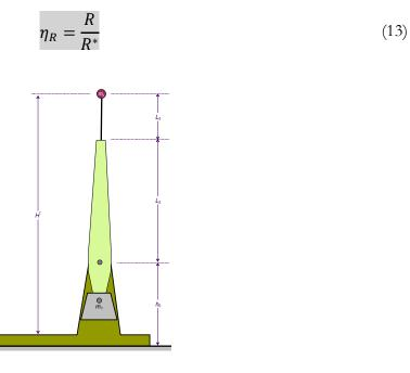
Note, however, that the launch height might not be the best that is achievable with a given trebuchet. The *maximum* launch height is obtained when both the arm and sling are vertical, and is given by
