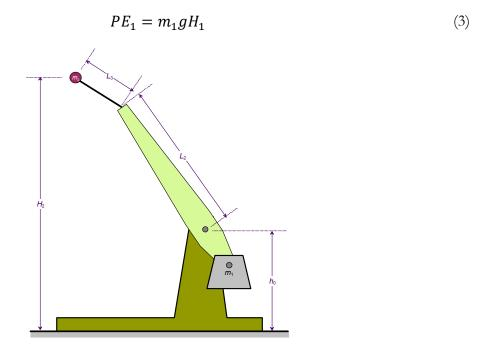
The projectile must be raised to its launch height, which uses some of the potential energy of the counterweight. As shown in the diagram above, the launch height of the projectile is
